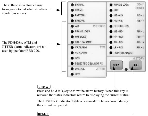
Press this key to reset the HISTORY store (all lit indicators extinguish). If an alarm condition is present during the reset, then the indicators associated with that alarm will remain lit after the reset. The resetting of the HISTORY store also occurs when you start a new test period. **Introducing Smart Test**
